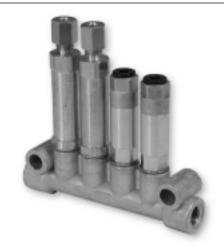
Positive Displacement Units (PDU's) deliver a precise volume of lubricant at the beginning of each pump cycle. Each unit in the range is stamped with a reference number denoting the discharge volume. The total oil delivery to a system can be further controlled by the pump lubrication frequency. The system operates intermittently, allowing PDU's to recharge for the next cycle, and is generally total loss.
